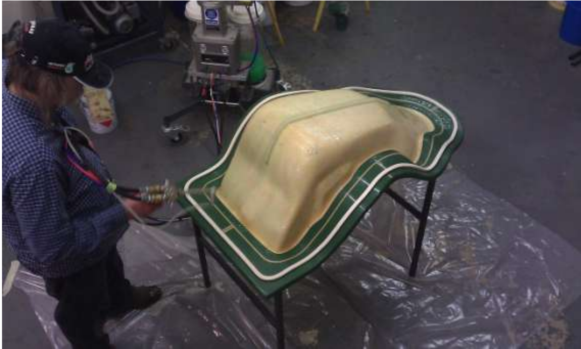
Figure 4 Silicone bag production by spray application
